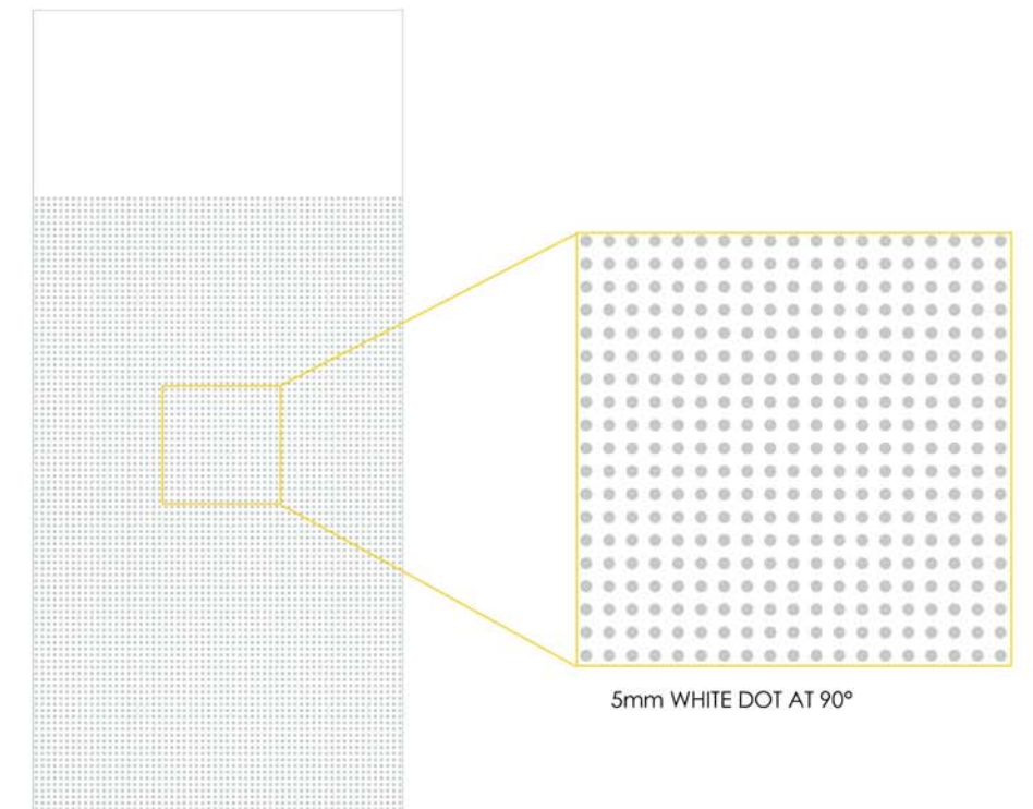
TYPICAL BALUSTRADE ELEVATION
